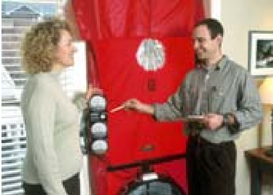
A certified Green$aver Advisor conducts blower door test
