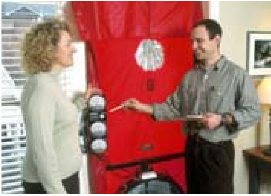
A certified Green$aver Advisor conducts blower door test
